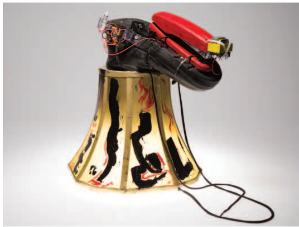
Fig. 1. The Boot , an absurd wearable electronic instrument made from assemblage of a boot, a black stapler painted red attached to the sole, a power coil and a lampshade, 2017. It generates sound by detecting electromagnetic fields that disrupt the operation of a simple built-in oscillator. (© Neal Spowage)
